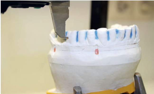
Fig 1 Measurement of the turning point.
